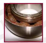
In similar studies at the same test facility, USC was able to demonstrate the survivability of AH-64 tail rotor drive shaft hanger bearings, often in **extremely** faulted conditions. The results of these experiments make it easier to identify faulted bearings without performing costly inspections and allow them to
